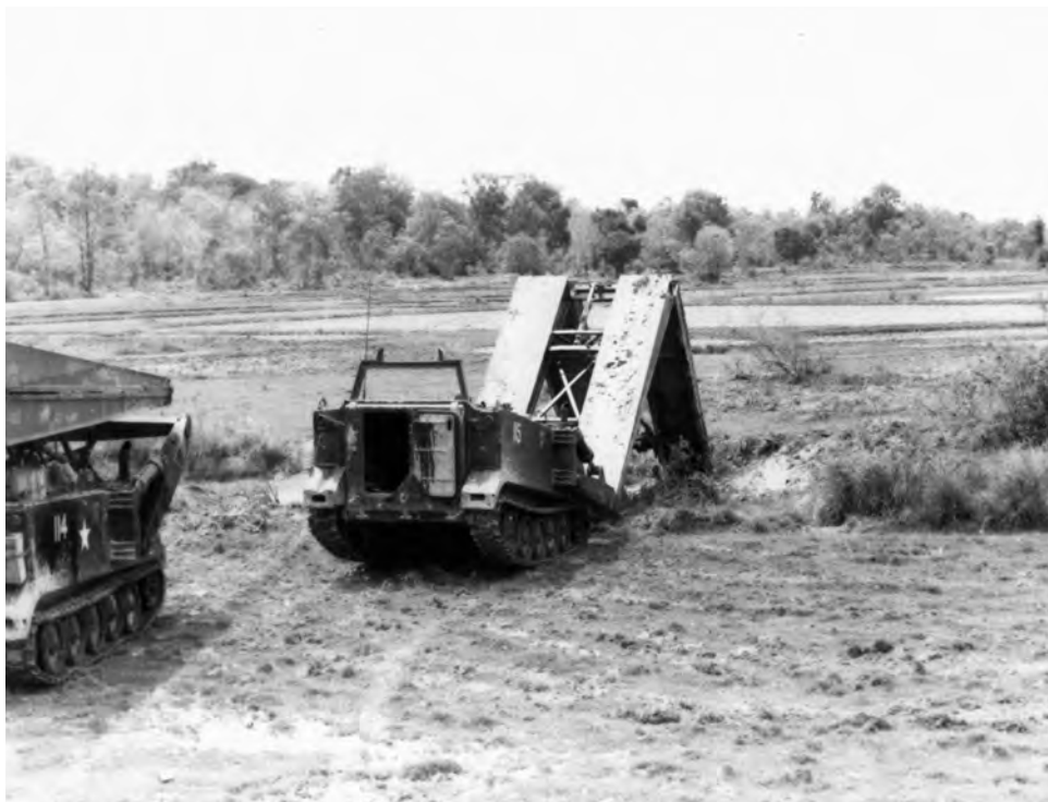
An armored vehicle launched bridge being emplaced in the Fishhook area of Cambodia
